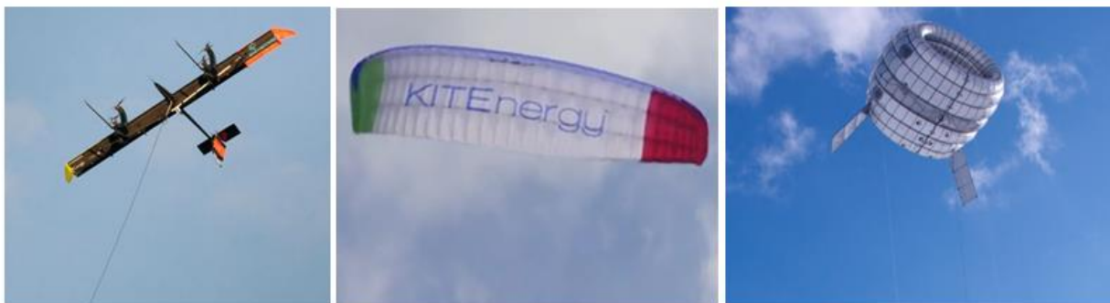
Figure 1: Recent airborne wind energy systems, including (left to right) the Makani Power (now owned by Google) M30 [11], KITEnergy KE60 [6], and Altaeros Energies Buoyant Airborne Turbine (BAT) [9]. A summary of airborne wind energy technologies can be found in [12].
